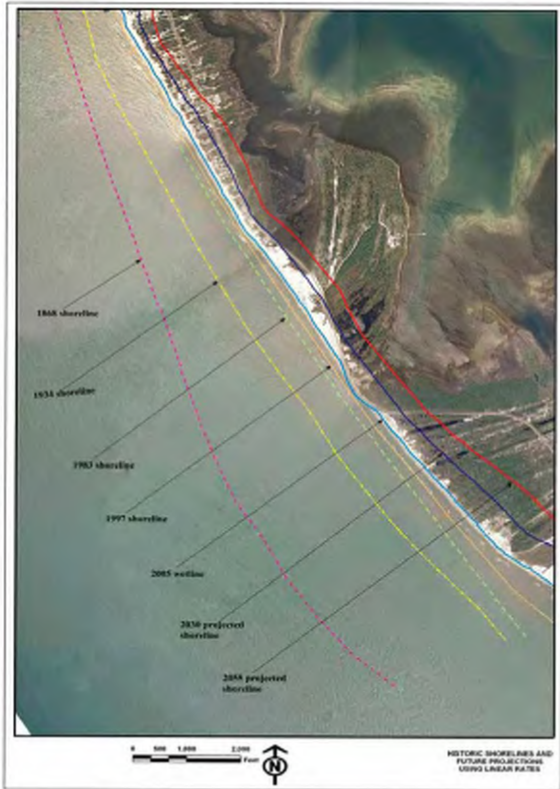
Figure 7.9. Example of projected future shoreline positions at Stump Hole (FDOT figure)
