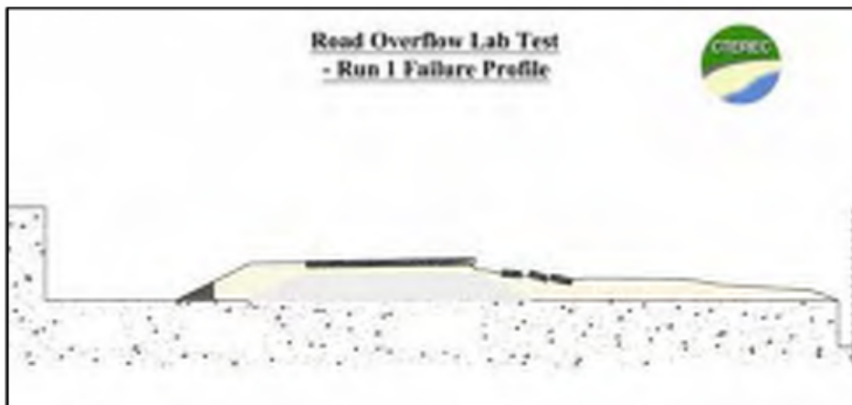
Figure 8.10. Schematic of USA/TAMU laboratory experiments test run one result
