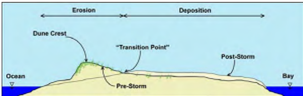
Figure 8.16. Schematic of sand erosion and deposition on a barrier island resulting from overwash.
